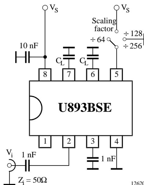
$C_L =$  Total capacitive output load including test fixture and test equipment capacitance
